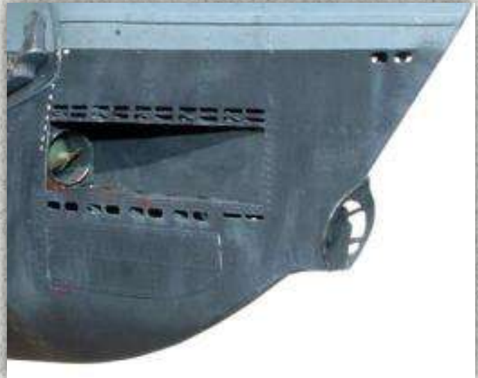
Above (H3): The S-Gerät bow device on the stem of U 557. The white markings are the waterline indicator decals (available from AMP).
