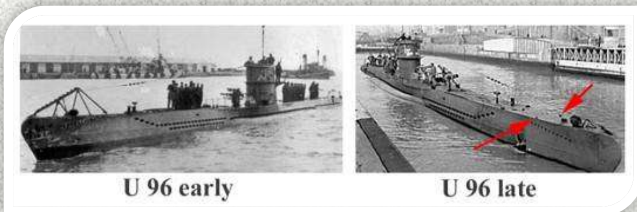
Above (C13a & C13b): The photo on the left shows U 96 with a net cutter. The photo on the right shows U 96 after the net cutter had been removed. The red arrows point to two of the triangular attachment points which were left at the edge of the deck when the net cutters were removed. There would be five brackets in total left upon removal of the net cutter.
