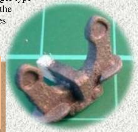
Right (H7): Powdered graphite was added to black paint to improve the look of the cast alloy anchor. The anchor recess was moved forward by 10mm.
