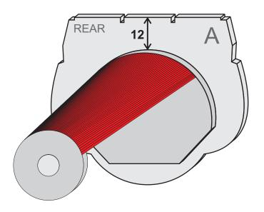
Glue the entire 'Stern' assembly to the <u>rear</u> of bulkhead A, so the top center of rib 'Stern-A' is 12mm from top of the bulkhead.
