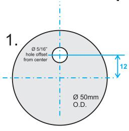
1. Cut 50mm disk from 0.080" plastic. Drill 5/16" hole offset from center by 12mm as shown.
