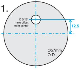
1. Cut 57mm disk from 0.080" plastic. Drill 5/16" hole offset from center by 12.5mm as shown.
