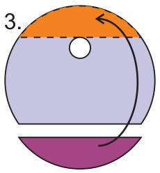
Glue the previously-cut segment to the other side as shown, edges flush.
