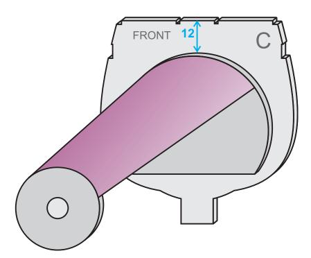
Glue the entire 'Bow' assembly to the <u>front</u> of bulkhead C, so the top center of rib 'Bow-C' is 12mm from top of the bulkhead.
